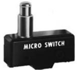
BZ Series Standard Basic Switch, Single Pole Double Throw Circuitry, 15 A at 125 Vac, Overtravel Plunger Actuator, 2,5 N - 3.61 N [9 oz - 13 oz] Operating Force, Silver Contacts, Screw Termination, CE, CSA, DEMKO,
